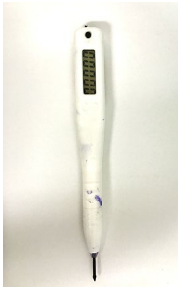
Figure 4 The counting incision device (Cole instruments) used to determine the number of follicles with regenerated hair.
